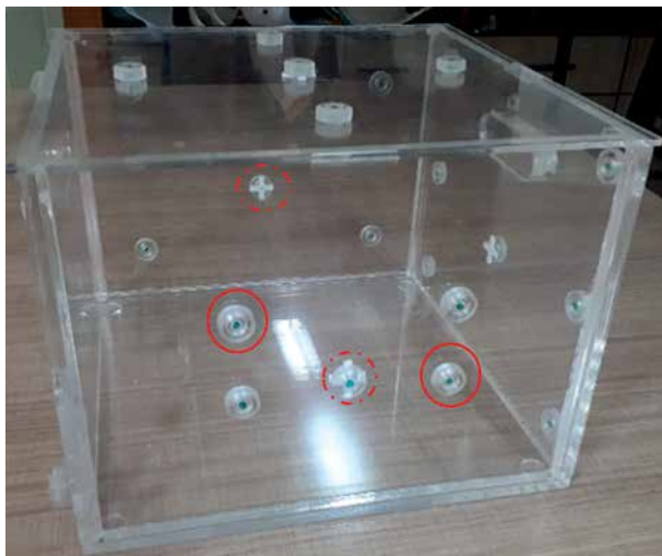
Fig. 4. Component P0: A waterproof box with 28 vitamin E markers for CT and MRI registration purposes (solid circles) and five cross hairs (dot circles) for aiding to align the P3 center with iso-center of CT and MRI scanners
