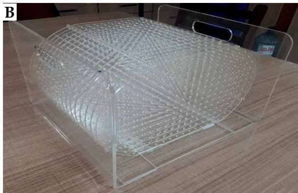
Fig. 2. A) The construction overview of component P2 for validating volume calculation accuracy; B) The component P3 with 17 parallel plates, each including 254 holes as control points for quantification of MRI distortion induced by MRI scanner
