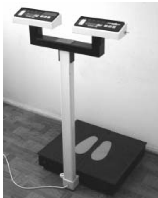
Figure 3. Electronic balance specially constructed for this research
