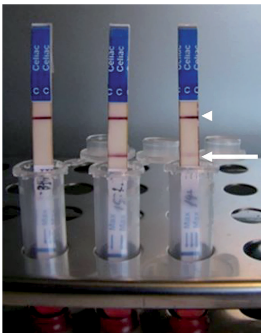
Figure 1. Positive and negative results for anti-transglutaminase antibodies using the rapid immunoassay. The first band (head-arrow) must always appear as a technical control, the second band (arrow) represents the positive result of the test. No second band was detected in the first strip incubated with a blood sample that tested negative for anti-transglutaminase antibodies. Different shades of grey bands identified coeliac patients in the second and third strip
