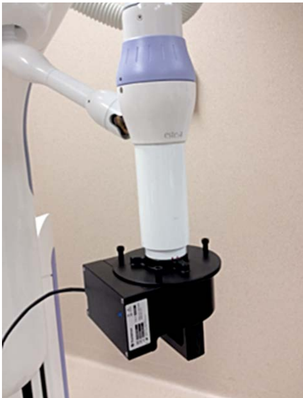
Fig. 4. Esteya unit with the QA tool provided by Elekta, which is composed of 26 diodes placed in two parallel planes in order to check constancy of output, flatness and PDD
