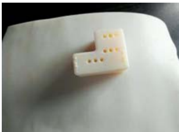
Fig. 5. 3D printed mold with preset needle pinholes. The mold has fixed channels for the needles and was 2 cm thick
