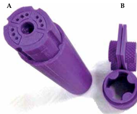
Fig. 2. Prototype of novel IMBRT applicator A) applicator with a diameter of 35 mm and B) auxiliary fixation tools
