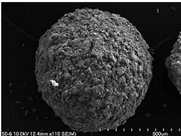
Fig. 1. Scanning Electron Microscope (SEM) image of composite granule with diameter of approximately 600 \mu\text{m} (magnification 110 \times )
